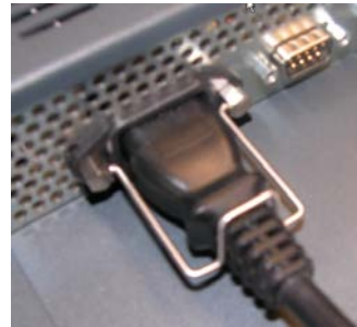
Power Cable Retention Clip Installed
